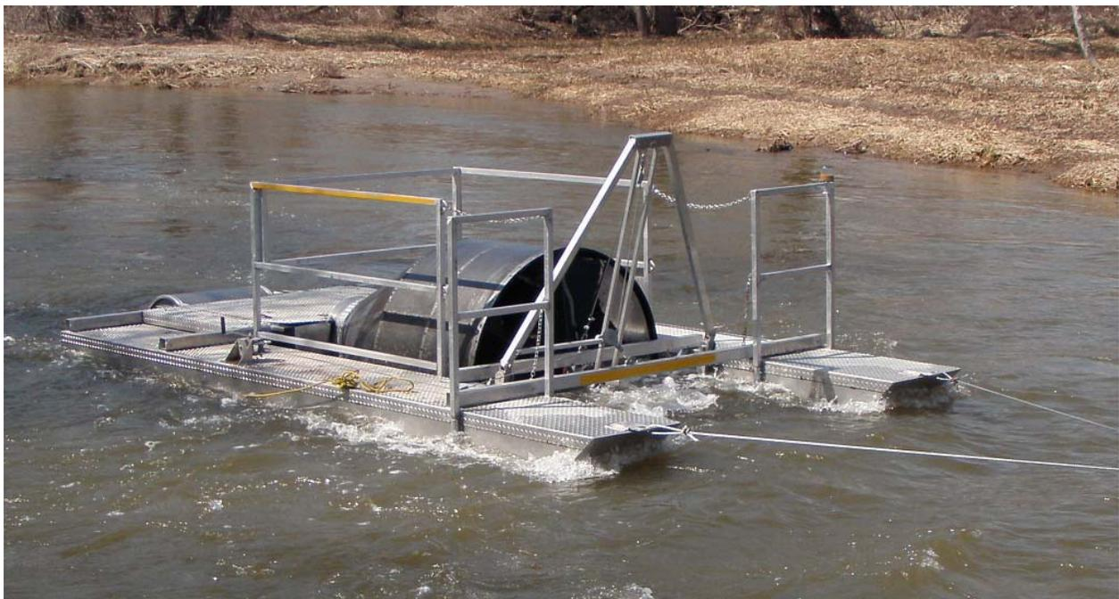
FIG. 2.9.1. Rotary Screw Trap at the Meadowvale Conservation Area on the Credit River.
