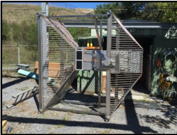
FIG. 1.12.1. VAKI Riverwatcher fish counter and frame custom designed for the Ganaraska Fishway.
