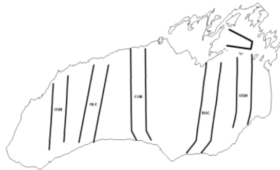
FIG. 1.6.1. The Lake Ontario Lake-wide prey fish survey uses cross-lake hydroacoustic transects. Transect corridors are logistically constrained but utilize a random starting point within the corridor for each annual survey.
