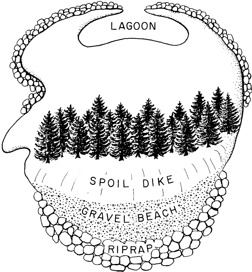
FIG. 6. Example of diked island-possible surface structure design.
