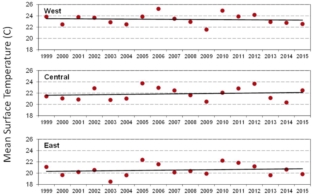
Figure 1.0.2. Mean summer (June-August) surface water temperature (°C) at offshore stations, by basin in Lake Erie, 1999-2015. Dark blue lines represent time-series average water temperature (1999-2012). Data included in this analysis by basin and station: West - 3, 6; Central - 8, 10, 11, 13; East - 16, 18, 19, 25.
