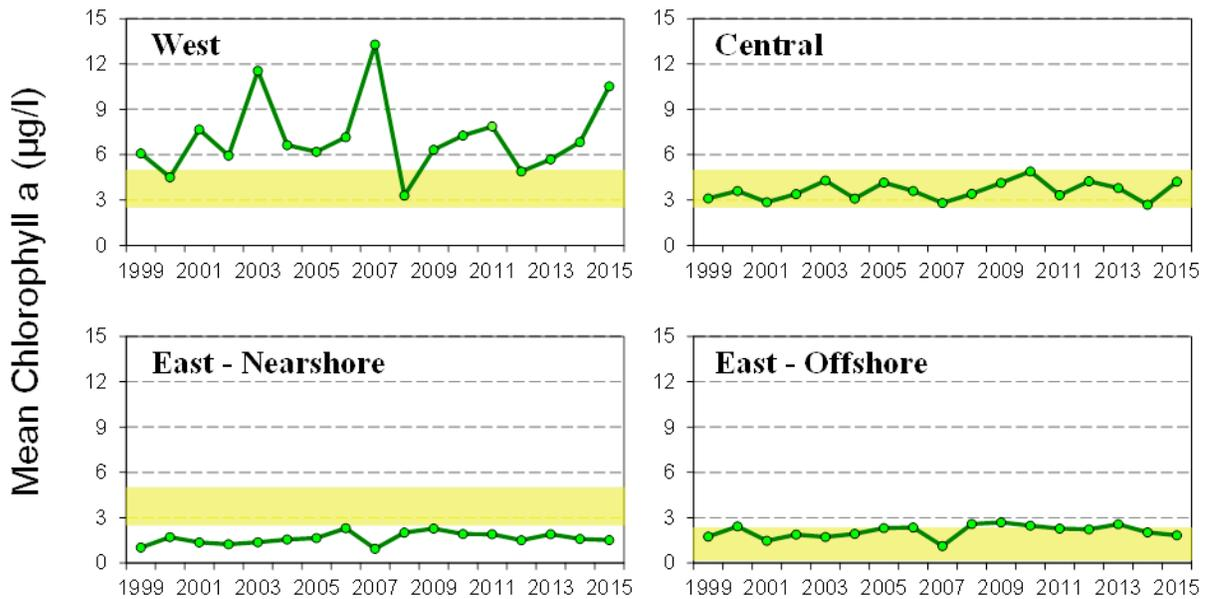
Figure 1.0.4. Mean chlorophyll *a* concentration ( $\mu\text{g/L}$ ), weighted by month, by basin in Lake Erie, 1999-2015. The east basin is separated into nearshore and offshore. Yellow shaded areas represent targeted trophic class range. For this analysis data from stations 3 through 20, and 25 were included.
